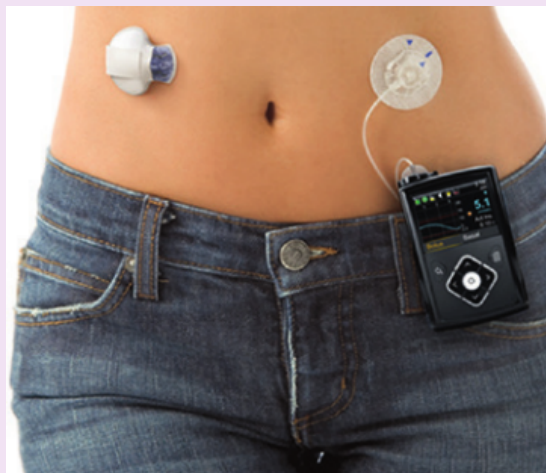
FIGURE 5-12 External insulin pump. The device on the patient’s right side is an insulin sensor which continuously monitors insulin levels and communicates with the insulin pump. (Provided by Medtronic.)
